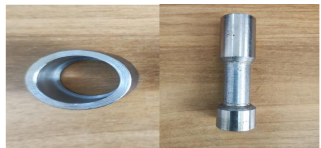
Fig. 2 Laboratory Press Die and Forming Mold Assembly for Briquetting
